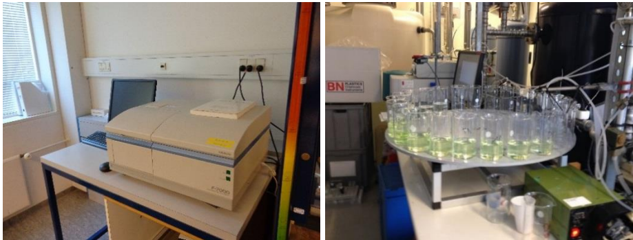
Figure 2.13: Lab spectrophotometer (Hitachi F-7000) and sampling carousel, which took samples of the pumped water at predefined intervals.
