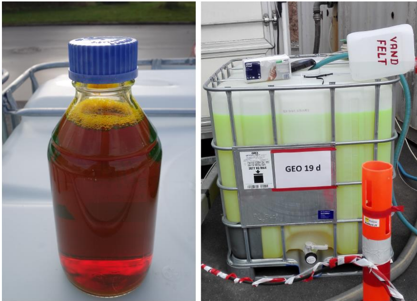
Figure 2.10: Concentrated fluorescein solution (left). 1000 L tank with diluted fluorescein (20 mg/L) and lithium bromide solution (1000 mg/L) before injection at borehole Geo19d (right).
