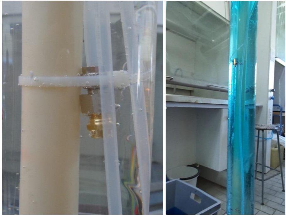
Figure 2.11: Lab test of the injection system. Tube with nozzle (left), candy dye injected into the plastic column showing a good mixing behavior (right).
