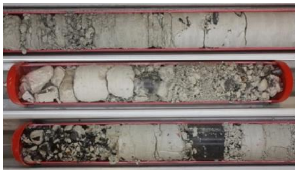
Figure 1.6: Borehole core samples from previous investigations (Geo4 and Geo9) showing crushed and fractured limestone with flint inclusions. Note that most of the fractures seen in the core samples were caused by the drilling.
